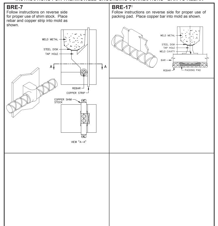
† Depending on weld type and rebar size, mold may go around or be placed onto rebar.
